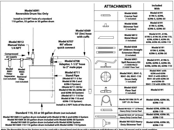
Note: The Reversible Drum Vac System must be used with a closed head steel drum with a minimum wall thickness of 1.3mm (18 gauge) and in good condition.
