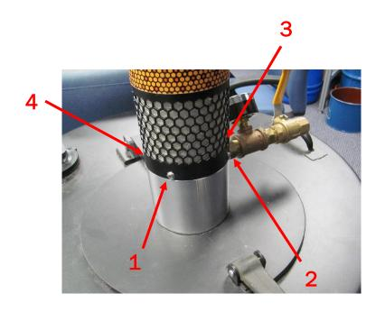
With a 1/8" hex allen key, remove (4) screws around bottom
